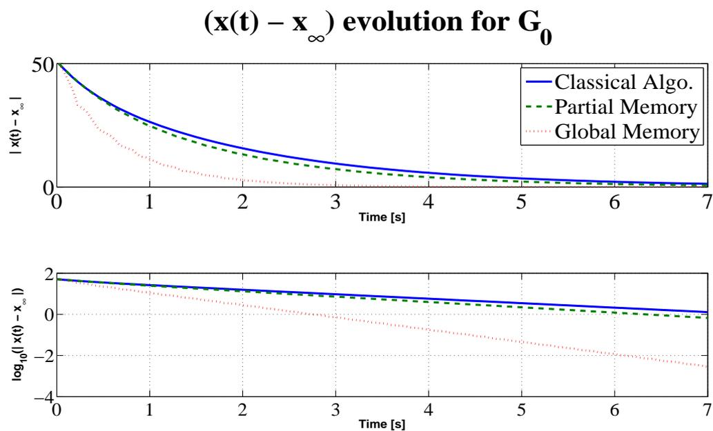
Figure 3.13: Time evolution of error  $\varepsilon_{SI}$  and  $\log_{10}(\varepsilon_{SI})$  for a set of six agents: performances comparison between (3.2.5) and (3.2.22) under a communication graph  $G_0$ .
